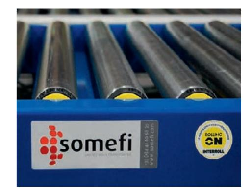
Rolling On Interroll: The conveyors used by Somefi are driven by RollerDrive made by Interroll.
