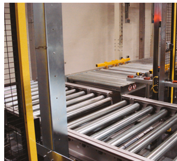
System throughput was increased to a level of 3,000 boxes per hour.
